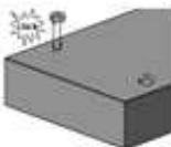
3. Put the mains cable through the hole in the casing.
